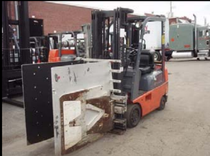
2004 Toyota 7FGCU18, cap 3500 lbs Mat 3 sections 83-189" Carton Clamp
